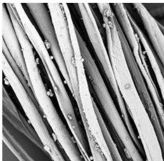
**Figure 3:** Fibres from the yarns made from the highest possible production rate
