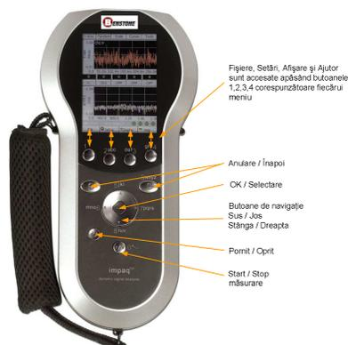
Vibration analyzers include a data analysis software that is installed on the PC. Program allows downloading and analysis of data performed by software modules installed in the vibration analyzer. It also has functions for post processing data, simultaneous viewing of several types of diagrams and spectra, making mathematical relationships (+, -, \*, /), integration, derivation, etc. Real-time filters. [6]
