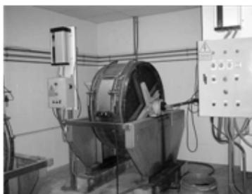
Figure 3. Tanning drum used in tanning tests on a semi-industrial scale
