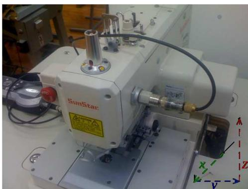
Figure 4. SunStar buttonhole machine with measuring vibration sensor installed on the axial direction
