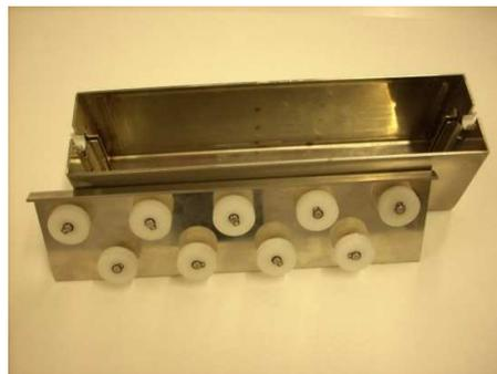
**Figure 1:** Device for the application of microcapsules on a core yarn
